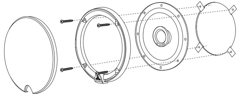
It is absolutely vital that the speaker frame fits into the mounting hole cleanly. This must be checked prior to tightening the screws. Do not force the frame into a hole that is too small! Do not tighten the speaker onto an uneven surface! This will damage your speakers. The speaker should also fit so that no air leaks around the mounting flange. Air leaks will cause a severe degradation in sound quality. Seal any air leaks with silicone, rope caulk or similar sealant material.
